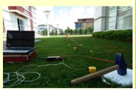
The DoReMi seismograph is an innovative instrument which distributes along the cable all the electronics needed to record a seismic signal.
